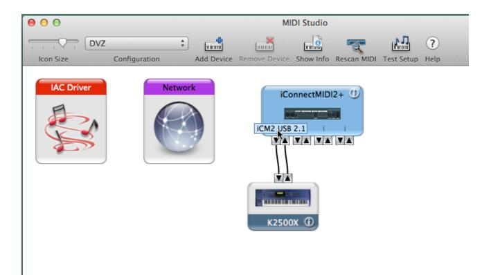
2. (Optional) In Audio MIDI Setup, create and cable connected MIDI hardware devices to the iConnectMIDI<sup>2+</sup> MIDI DIN ports.
