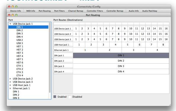
Bear in mind that jacks are physical connections and ports are 16-channel MIDI ports; one jack can carry several ports. For example, each USB Device jack has 16 MIDI ports.
