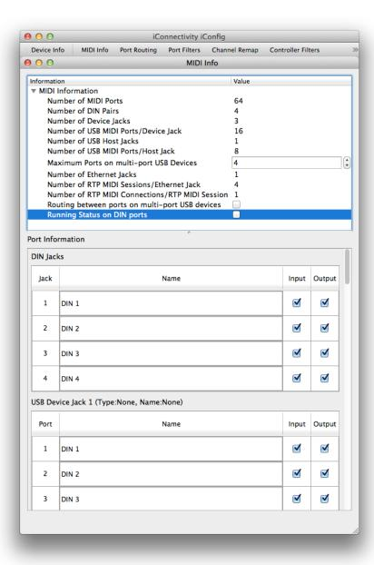
About the "Running Status on DIN ports" checkbox (under MIDI Information): this defaults to being disabled/not transmitted (white), since it must be implemented – and implemented correctly - in the receiving device to function. As a practical matter, Running Status is a "leave it off unless you know otherwise" parameter.
