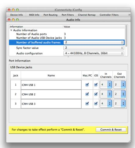
Audio Configuration: this drop-down in the Audio Information window offers a choice of seven different combinations of sample rate, number of audio channels, and bit rate. (Audio channels are divided evenly between input and output.)
