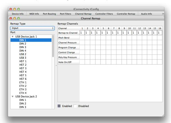
Then go over to the Remap Channels table and select the data type and channel to be remapped, and enter the destination channel number in the Remap to Channel row.
