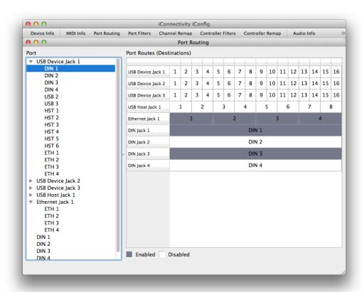
There are countless applications in which the routing feature might be useful. Perhaps you need one MIDI keyboard controller routed to a layered sound that's on two different computer devices, or maybe you have a percussion pad that you want "hardwired" to a percussion module. Or perhaps you don't need the computer device connected to iConnectMIDI<sup>4+</sup> USB jack 1 to see the MIDI keyboard connected to DIN jack 1.
