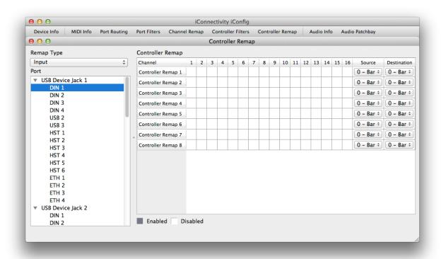
Then choose the Controller types in the Source and Destination dropdowns on each row, and enable/disable the MIDI channels you want the conversion to apply to. The lists of available controllers are identical to the one in the Controller Filters tab above.
