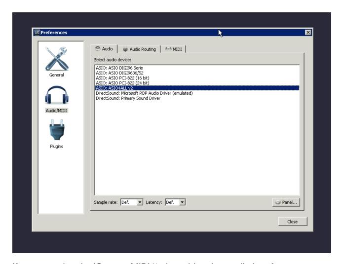
If you are using the iConnectMIDI4<sup>+</sup> alongside other audio interfaces installed on the Windows computer, as shown above, they are automatically "aggregated" into what appears to the software as a single interface with combined number of outputs in each one.
